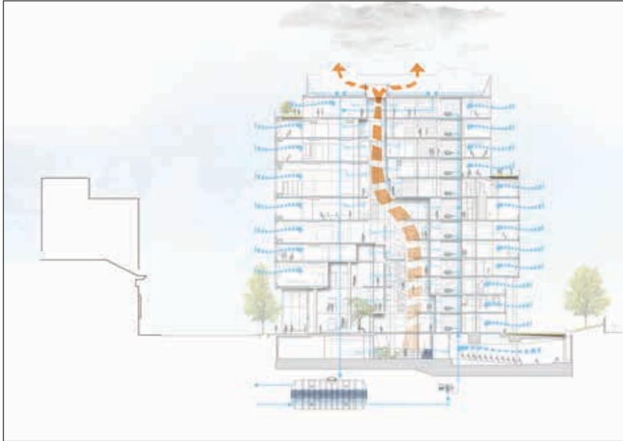
The full-height atrium serves as the ventilation pathway for the entire building. Five high-capacity exhaust fans at the top can supplement the automated natural ventilation system.
